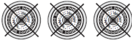
improperly loaded rotors
